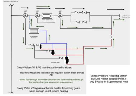
VT has an inlet orifice of a fixed diameter ('no moving parts'), plurality of the VT provides for operations in a broad range of fluctuations of the VPRS inlet flow. Each VT has an upstream control valve (CV) that senses the delivery pressure downstream of the VT. Each CV has a distinct set pressure within the station MAOP, such that each VT begins to supply sequentially as demand increases. Similarly, as demand decreases each VT stops supply sequentially.
